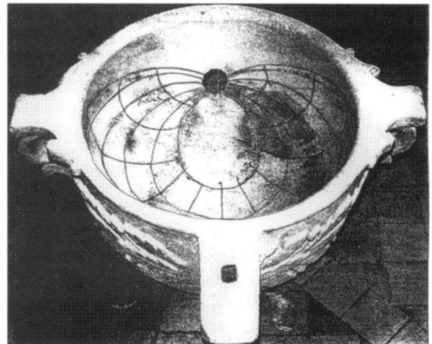
Fig.3b Photographs of the interior of the scaphe to show date lines and hour lines
